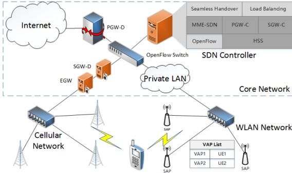
Fig. 1. The Convergence Architecture in LTE and WLAN
